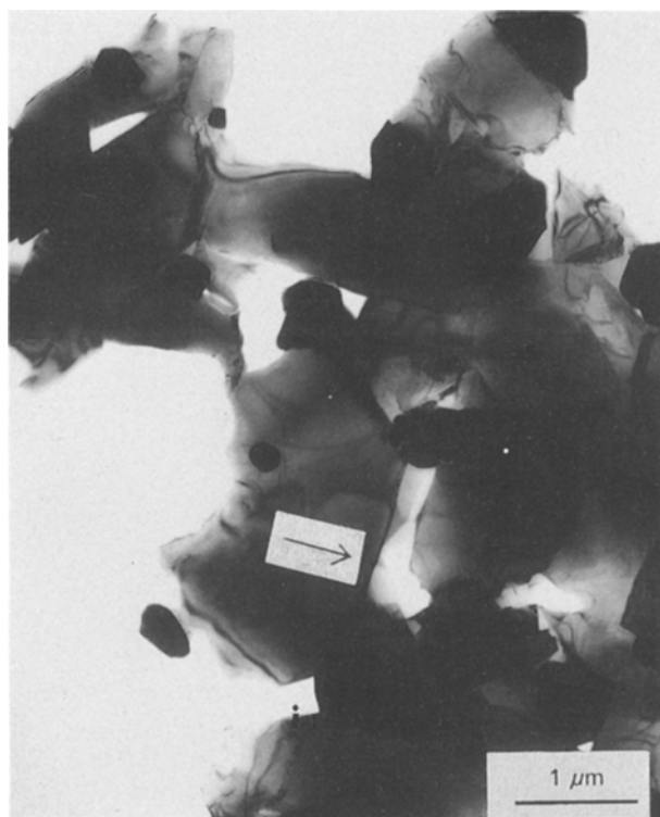
Figure 6 TEM micrograph of the composite hot-pressed at 1600°C in argon, showing an amount of SiO 2 left in grain boundaries of mullite.
