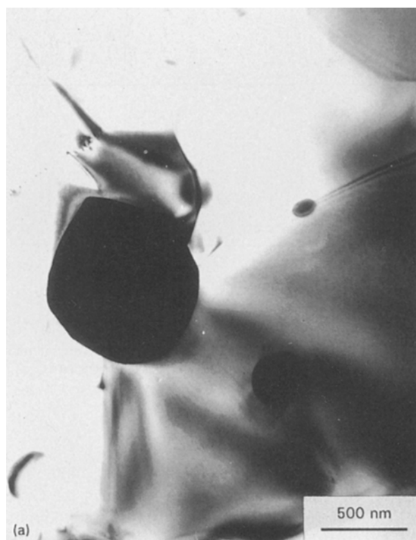
Figure 4 TEM micrographs of the composite hot-pressed at 1450 °C (a) in vacuum; (b) in argon, showing bright field image and appearance of dislocation, strain contour in the matrix; and (c) selected-area diffraction pattern (SADP) of Cr 3 C 2 phase with orthorhombic structure with zone axis [10 \bar{1} ].
